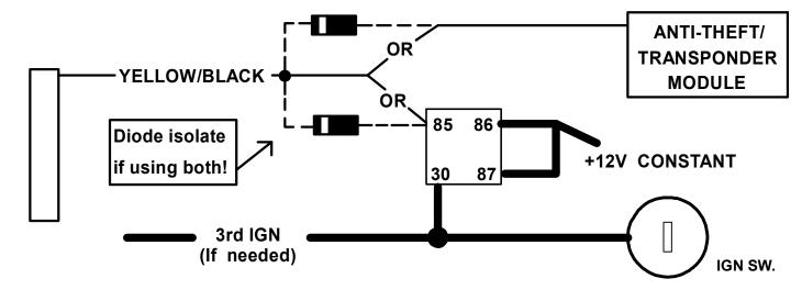
PIN 3: YELLOW/BLACK: FOR ANTI-GRIND/STARTER DISABLE OUTPUT: (Relay not included)
